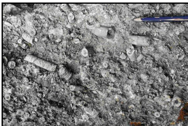
Figure 8: Crinoidal limestone, typical of shallow water back reef areas where the depositional environment is high energy, the lime mud is removed and the crinoid stems are left broken and sometimes aligned by strong currents. Stone Centre, Worksworth
